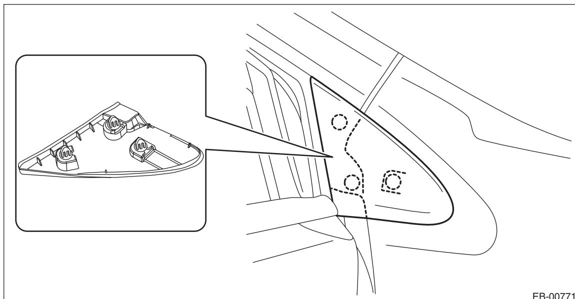
8) Remove the garnish assembly - fender. <Ref. to EB-21, FENDER GARNISH, REMOVAL, Front Fender.>
