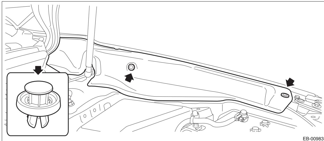
5) Remove the mud guard - front. <Ref. to EI-23, REMOVAL, Mud Guard.>
